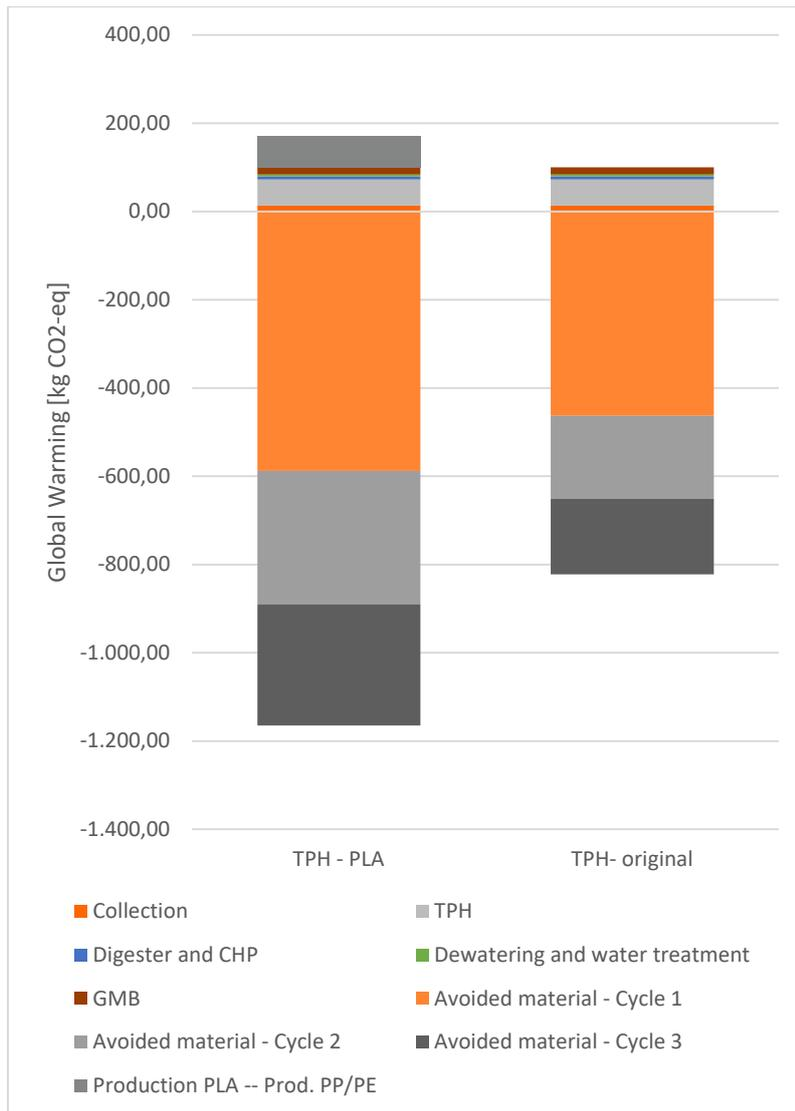
Figure 2 Contribution analysis by process steps in Global warming potential
